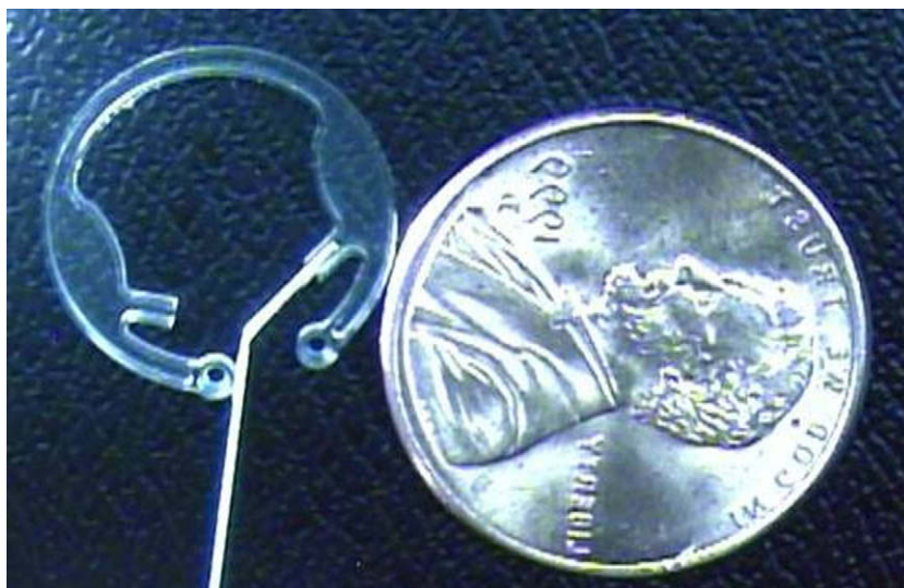
Fig. 3. The picture of a prototype prior to membrane and valve assembly with a 27 G cannula in the valve access port.
