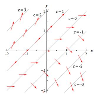
To add more arrows for those areas between the isoclines start at say, c = 0 and move up to c = 1 and as we do that we increase the slope of the arrows (tangents) from 0 to 1. This is shown in the figure below.
