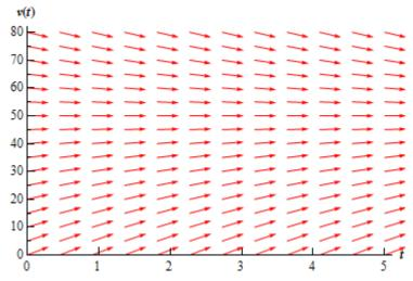
This graph above is called the **direction field** for the differential equation.
