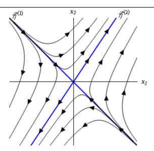
In this case the equilibrium solution (0,0) is called a **saddle point** and is unstable. In this case unstable means that solutions move away from it as t increases.
