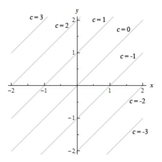
Now, on each of these lines, or isoclines, the derivative will be constant and will have a value of c. On the c=0 isocline the derivative will always have a value of zero and hence the tangents will all be horizontal. On the c=1 isocline the tangents will always have a slope of 1, on the c=-2 isocline the tangents will always have a slope of -2, **etc.** Below are a few tangents put in for each of these isoclines.
